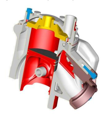
Aluminum cylinder head composed by an internal combustion chamber and an outher cover. Stiff and light
